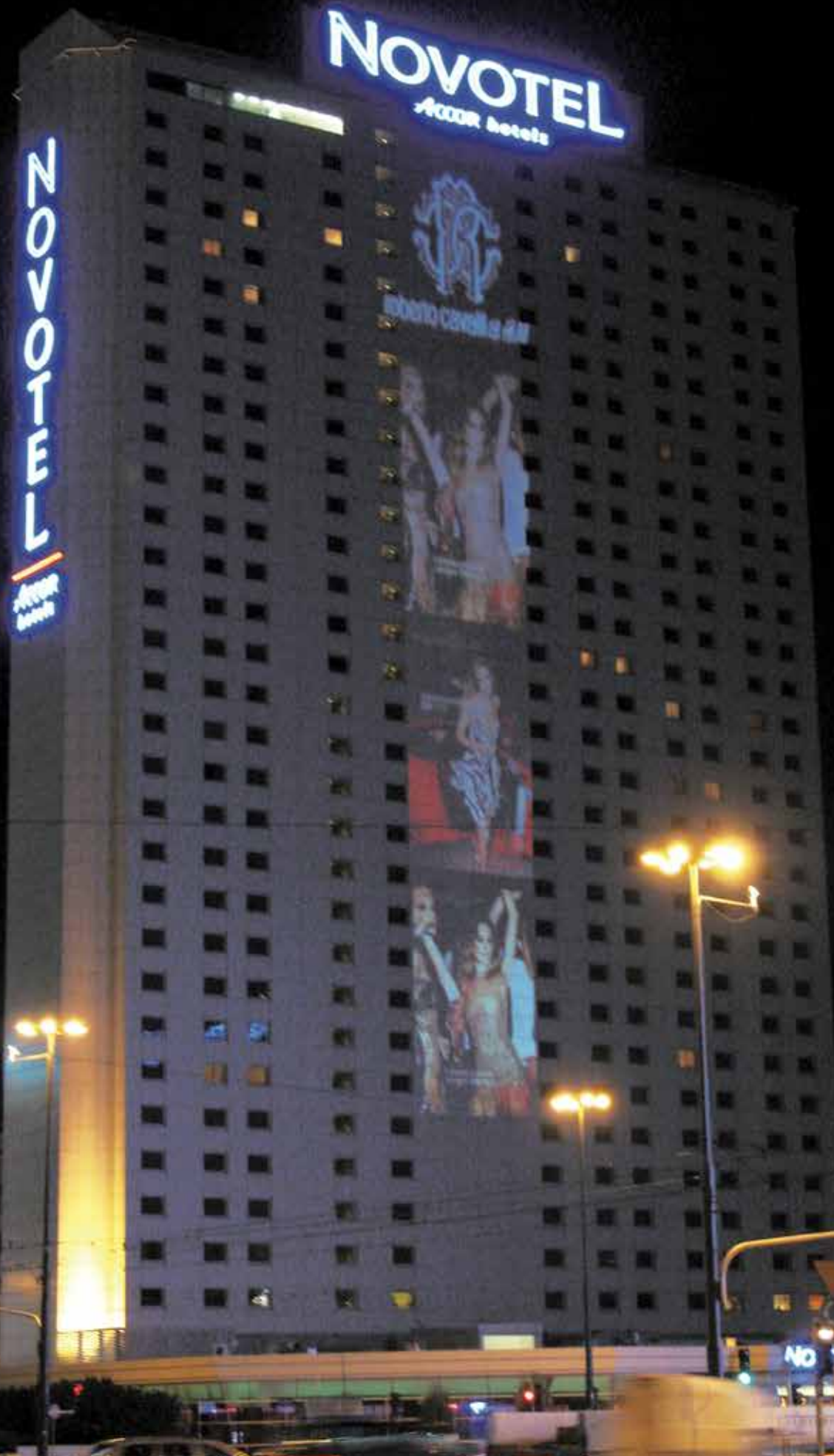
Photo: Projections made with 4 x 930 SNX profile spots - Image size: 18m x 10m each
